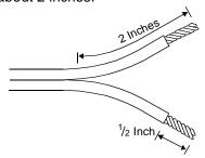
Strip the insulation from the ends of each conductor to expose <sup>1</sup>/<sub>2</sub> inch of metal wire, then twist the loose wire strands.
